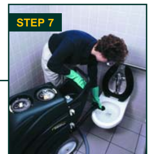
STEP 7 Empty recovered water into toilet, mop, sink or floor drain using the drain hose.
